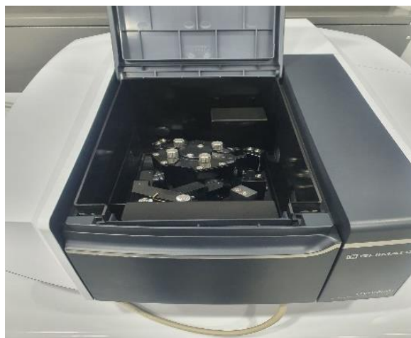
3-rasm. Diffuz aks etish spektrlarini olish uchun ISR-2600 integratsion sfera
